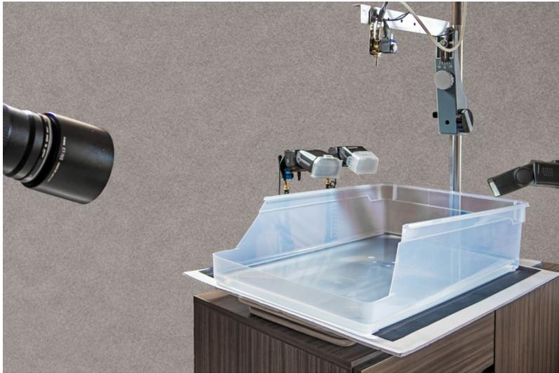
Figure 2 : The recording device for water drop photography
